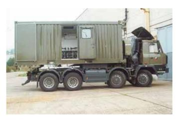
THE CONTAINER ISO 1C DRINKING WATER TRANS-PORTER (hereafter 'the container' only) is fully designed to be filled with drinking water, to transport it and to discharge it. Its maximal capacity is 8 m³ and is to be consumed in 24 hours. It secures the delivery of drinking water to the following: COOKER SET, SANITARY CONTAINER, FIELD HOSPITAL etc.
